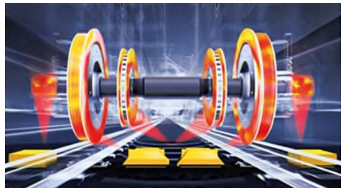
Hot bearing detector
