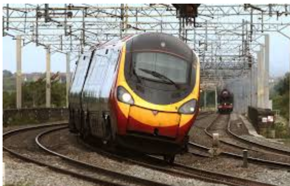
Cant track and tilting train
